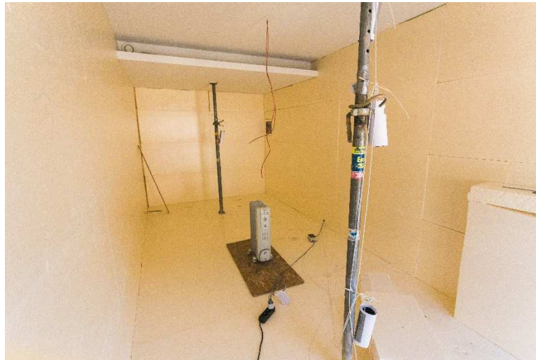
Figure 27 : Electric radiator in the insulated unit
