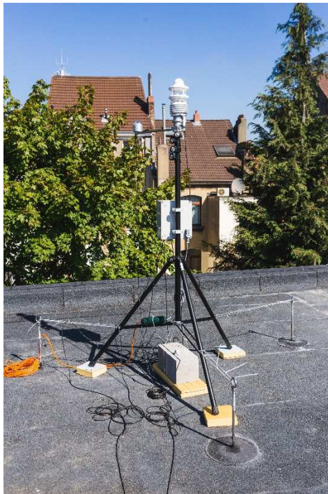
Figure 35 : Weather station on the roof
