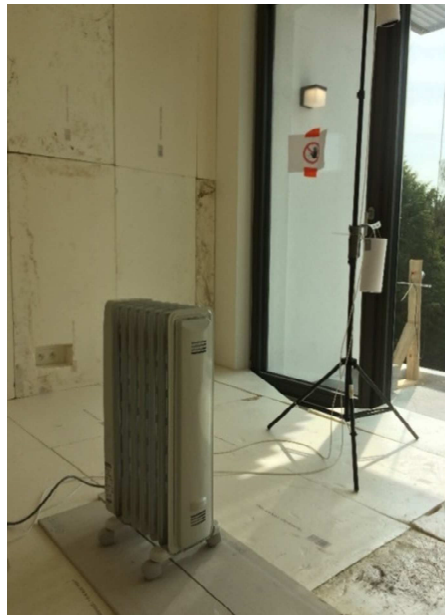
Figure 31 : Electric radiator in the insulated unit (living)
