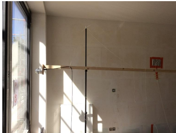
Figure 34 : Pyranometer in unit BU
