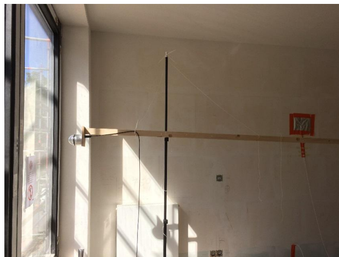
Figure 21: Pyranometer in front of the window in unit BU
