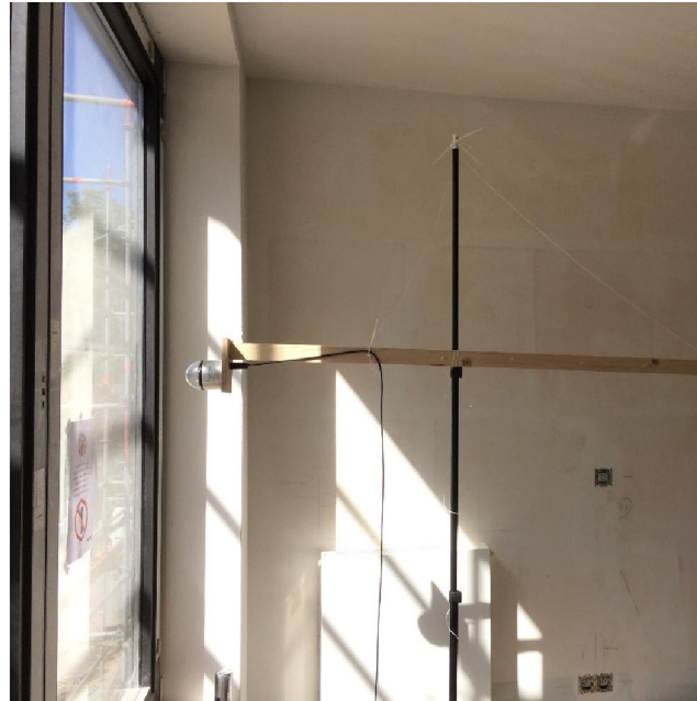
Figure 29 : Pyranometer in front of the window in unit BU
