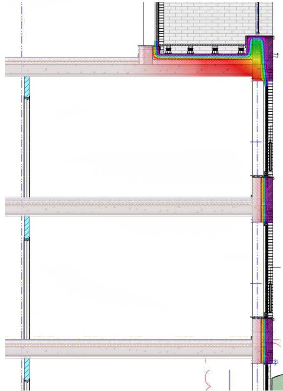
Figure 22 : Section drawing of the main thermal bridges
