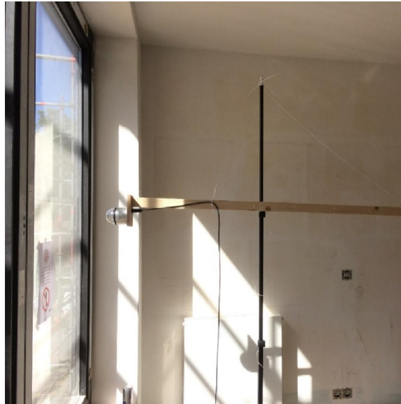
Figure 25 : Pyranometer in front of the window (picture taken from another experiment but the configuration was the same)
