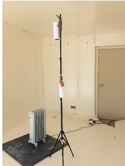
Figure 23 : Electric radiator in the insulated unit (AI)
