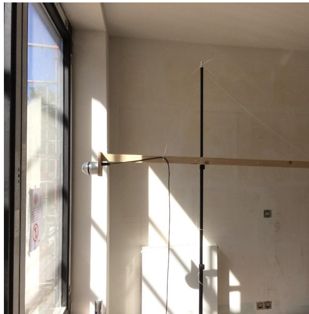
Figure 22 : Pyranometer in front of the window in unit BU
